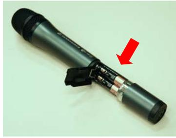
(Photo 2) Insert batteries
