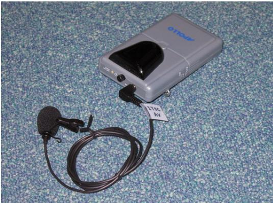
Connect the Tie-clip Microphone to the Transmitter.
